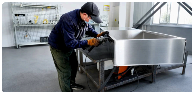
4 · Grinding Edges and welds ground smooth
