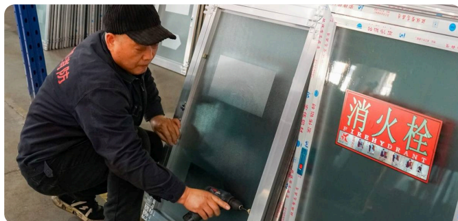
6 · Assembly Glass, hinges, locks and lettering fitted
