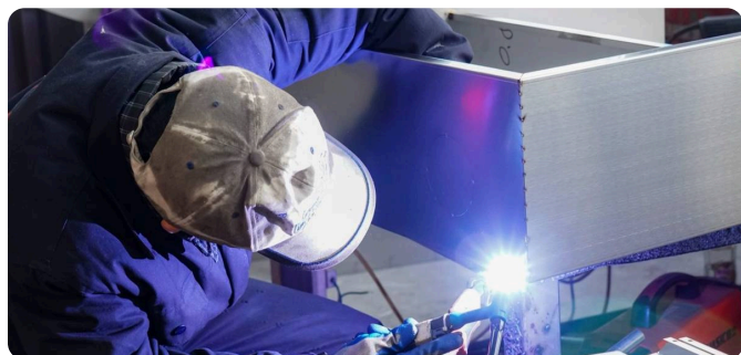
3 · Welding Body and door frames welded in-house
