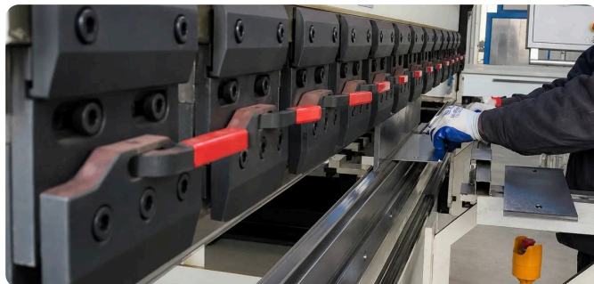
2 · CNC bending Body and door panels folded to drawing
