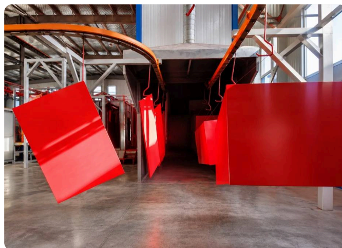
Automatic powder coating line
